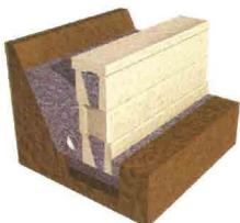
Lay the next course and subsequent courses to a string line following the same procedure, as outlined in Step 4, cleaning the top of the blocks, filling the block cores and backfilling behind the blocks to a maximum of one block high, at a time (as per Step 5).
