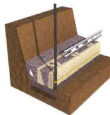
Spread 25mm of washed sand over the compacted base.
