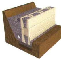
Place 100mm diameter PVC agricultural pipe with sock behind the wall, with a 1 in 100 fall. Backfill behind the courses of blocks to a width of approx. 200mm - 300mm using 10-20mm clean aggregate. Ensure each block is also well filled with clean aggregate.
