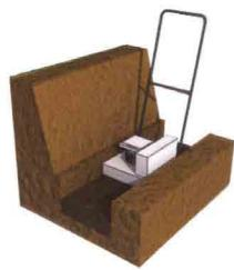
The subgrade should be compacted by several passes of a mechanical plate vibrator. Where there are significant variations of subgrade or compaction soft spots, or where there is ponding of ground water, the material shall be removed, replaced and compacted in layers as per engineer's advice. Trenches shall be dewatered and cleaned prior to construction, such that no softened or loosened material remains.
