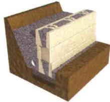
Place 100mm diameter PVC agricultural pipe with sock behind the wall, with a 1 in 100 fall. Backfill behind the courses of blocks to a width of approx. 200mm - 300mm using 10-20mm clean aggregate. Ensure each block is also well filled with clean aggregate.
