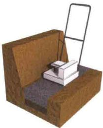
The facing shall be built on a base not less than 150mm thick, consisting of one of the following options:
